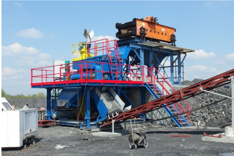
Fig. 1. K-102 No.2 pulsatory classifier built in the installation for a reclamation of extractive waste dump [7]
