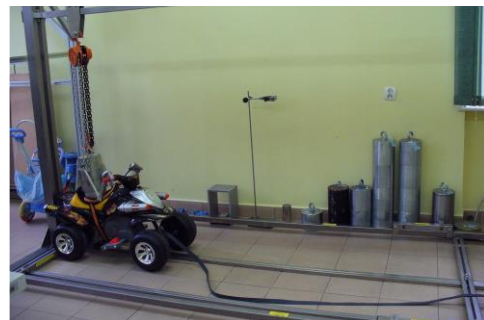
Fig. 5. Test rig for testing a safe use of products for children
