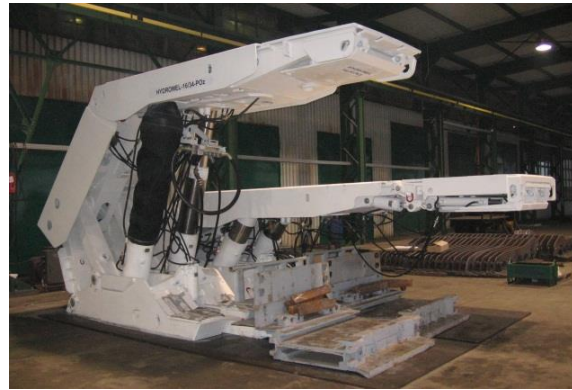
Fig. 14. HYDROMEL 16/34-POz powered roof support unit [14]
