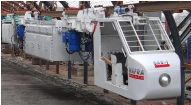
Fig. 6. Haulage unit of the GAD-1 suspended monorail [9]
