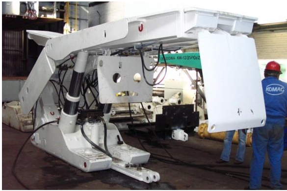
Fig. 13. KHW 12/28-POz/Pp powered roof support unit [14]
