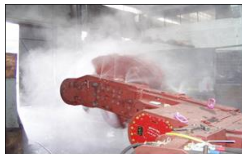
Fig. 9 Air-and-water spraying installation built in the RW-200N ranging arm of the KSW-460NE shearer [11]
