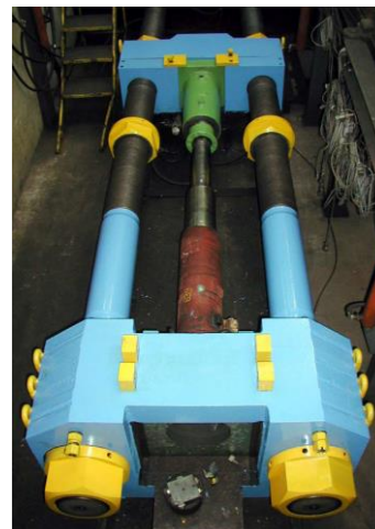
Fig. 2. A view of the rig for testing legs and elements of high pressure hydraulics for mining machines and equipment [3]
