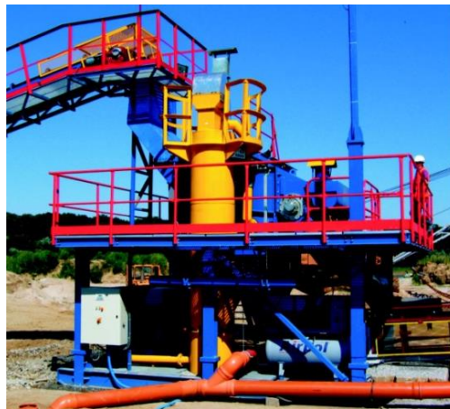
Fig. 17. Pulsatory classifier of dividing and separating organic and mineral impurities from natural aggregates [16]
