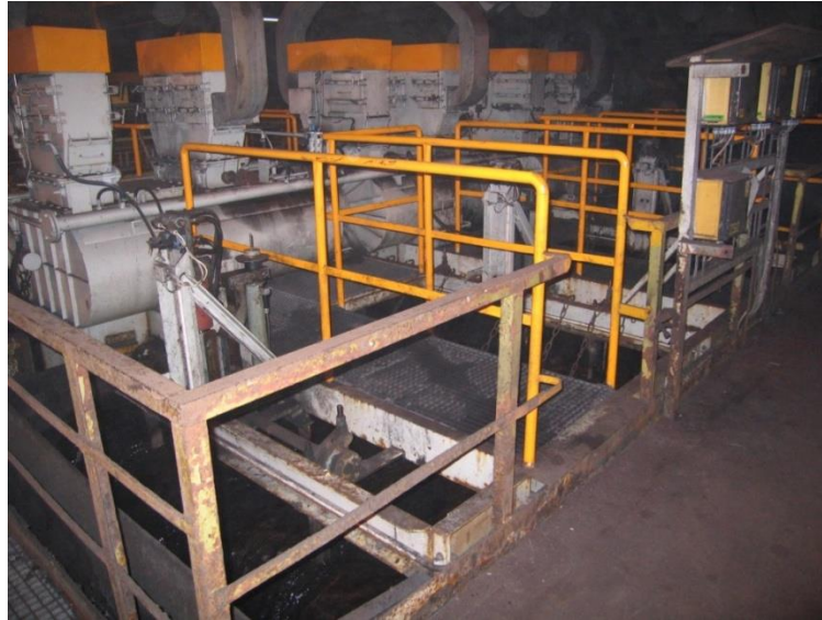
Fig. 1. OS26D3E medium-size-grain jig
