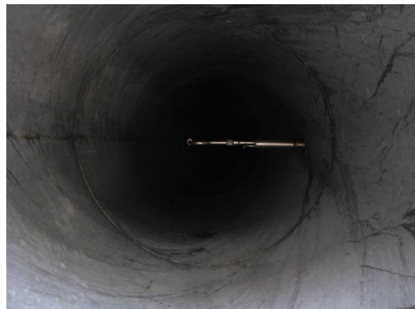
Fig. 2b. Measuring probe with the filter installed in the tested ventube pipeline
