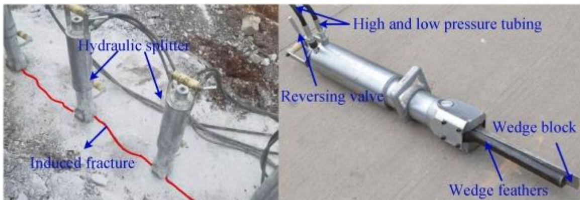
Fig. 8. Hydraulic splitter employed for the non-explosive fracturing of rock in engineering application [21]
