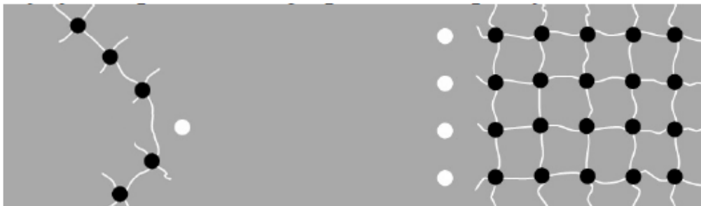
Fig. 10. Directions of cracks propagation in the rock block depending on the place of using the expanding materials [22]
