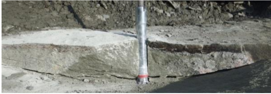
Fig. 15. Under-cutting bolt: method of the bolt fixation and range of loosening fracture propagation [20]
