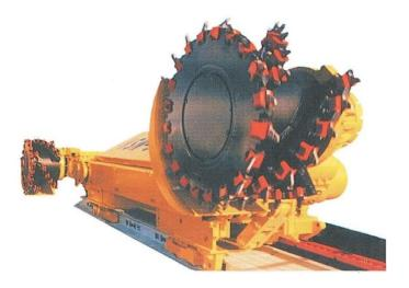
Fig. 14. KSE-500 longwall shearer [KOMAG]
