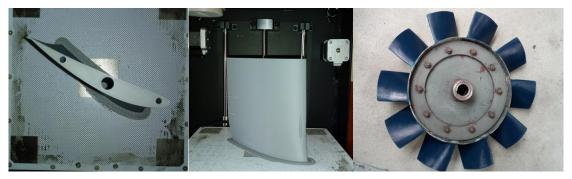
**Fig. 5.** 3D printouts of fan blades with space for reinforcing bars, the fan modified by adding prints changing the shape of the blades [11]
