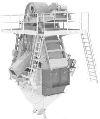
Fig. 17. DISA 2S suspension separator [10, 14]
