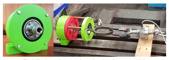
Fig. 4. 3D printout of the magnetic coupling, view of the test stand [10]
