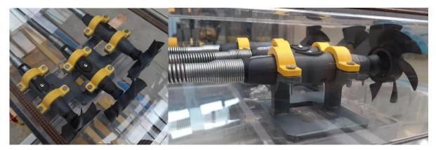
Fig. 6. 3D printed support brackets for the construction of the test stand
