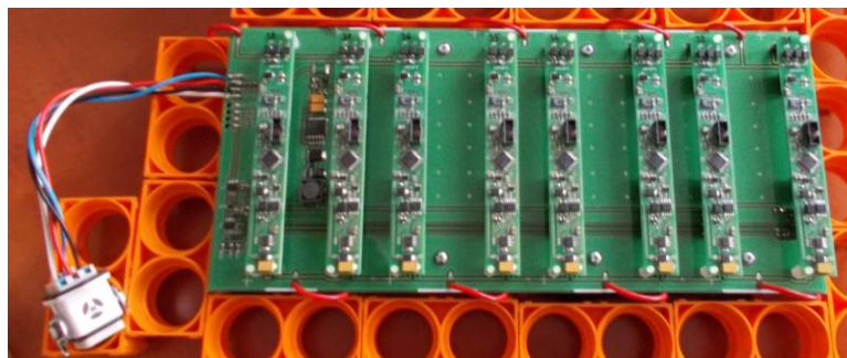
Fig. 7. BMS-S modules installed on the assembly board
