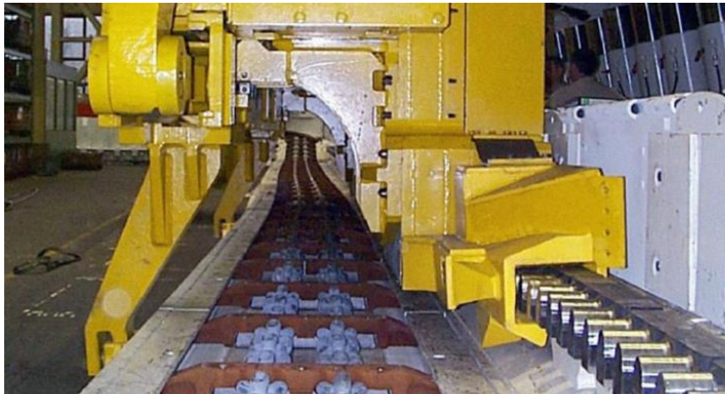
Fig. 4. The Saartrack chainless haulage system [7]
