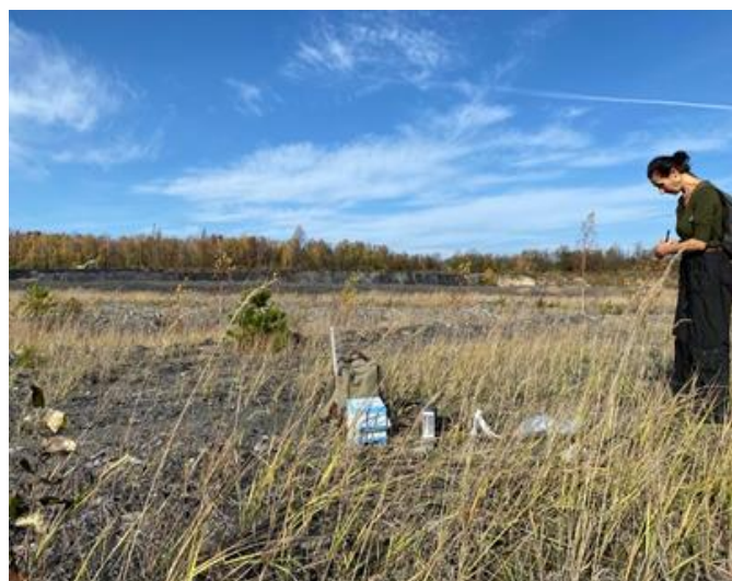
Figure 2.2.2. The soil respiration chamber enables the measurement of the short-term value of the CO 2 release. Along with respiration rate, the measurement of temperature and moisture of the spot where the measurement has been taken. The respiration rate can be expected to be varied, in different vegetation communities assemblies
