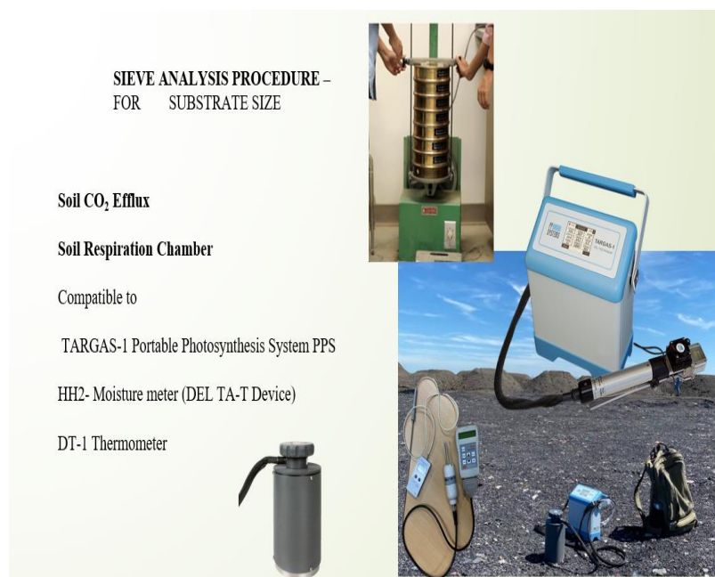
Figure 2.2.1. The equipment used for the measurement of soil respiration and the assessment of the texture of soil or soil substrate
