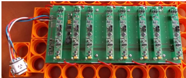
Fig. 7. BMS-S modules installed on the assembly board
