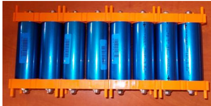
Fig. 4. Battery pack made of eight lithium cells
