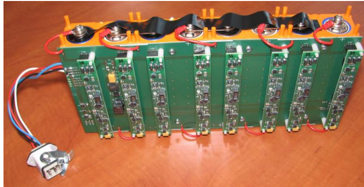
Fig. 9. BMS installed on the cells pack
