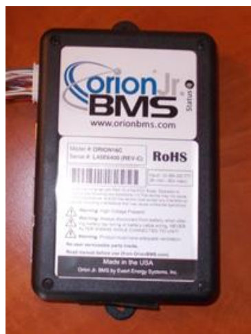
Fig. 5. System BMS ORION
