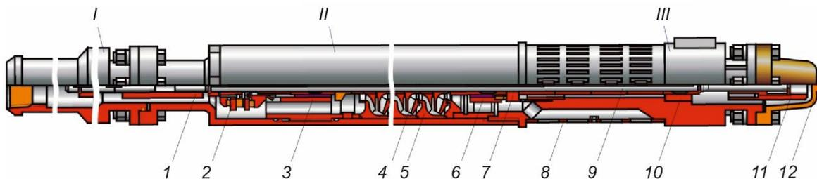
**Fig. 2.** Submersible centrifugal pump
