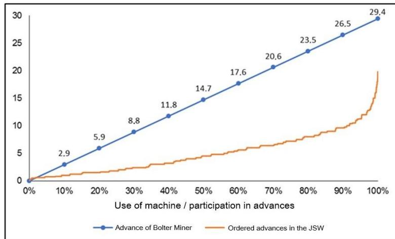
**Fig. 8.** Relationship between the working development advance and the degree of the 12CM30 Bolter Miner use in relation to advances achieved at JSW S.A. with use of conventional method of developing roadways with roadheaders
