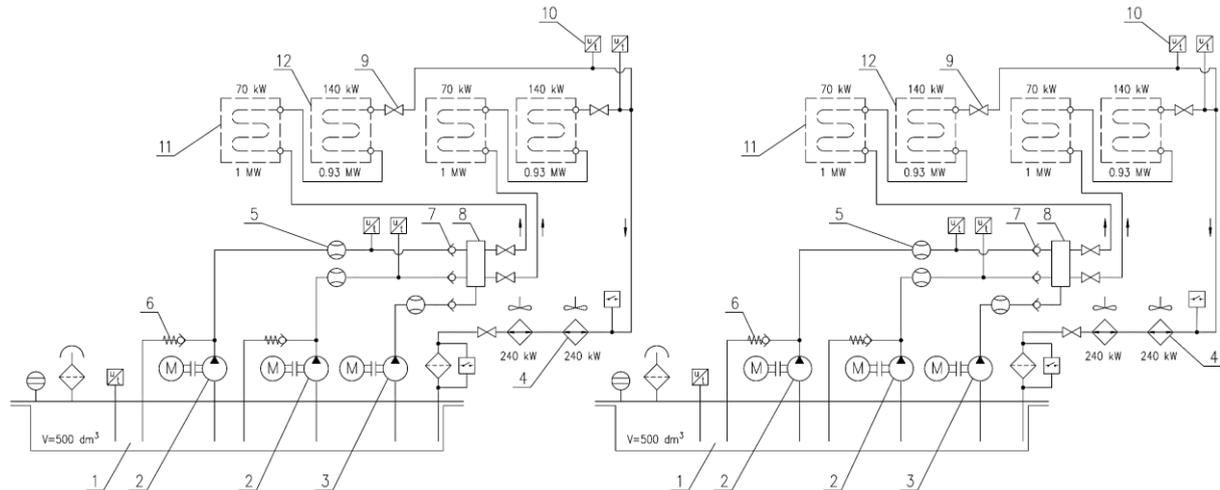
**Fig. 7.** Diagram of the surface cooling system of conveyor belt drives: 1 - tank, 2, 3 - pump units, 4 - air-water cooler, 5 - flow meter, 6, 7 - check valves, 8 - collector, 9 - cut-off valve, 10 - temperature sensor, 11 - electric motor flow system, 12 - gear flow system
