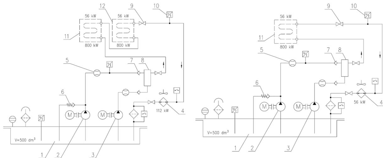
**Fig. 11.** Diagram of the cooling system of the underground drive with the use of a gear with higher efficiency: 1 - tank, 2, 3 - pump units, 4 - air-water cooler, 5-flow meter, 6, 7 - check valves, 8 - collector, 9 - cut-off valve, 10 - temperature sensor, 11 - electric motor flow system, 12 - gear flow system
