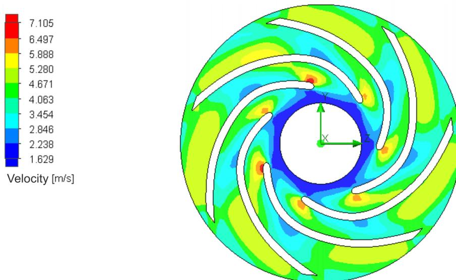
**Fig. 10.** Velocity distribution in the cross section of the impeller
