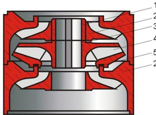
**Fig. 3.** Stage of a submersible pump
