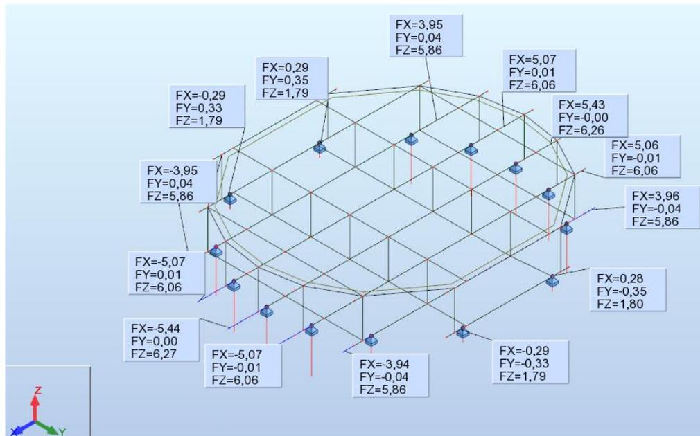
Fig. 8. Values of support reactions (units: kN)
