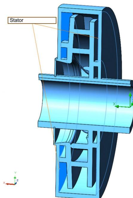
Fig. 8. Selecting model surfaces that should not rotate
