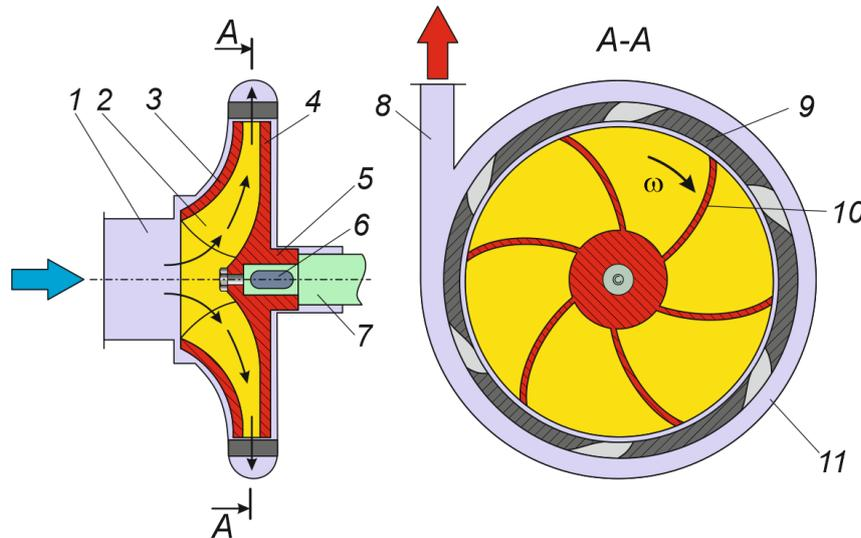
**Fig. 1.** Scheme of a sectional pump (one section)
