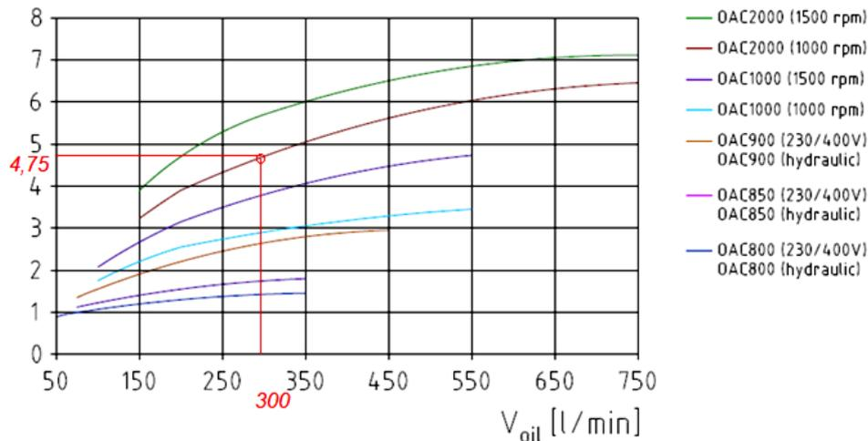
Fig. 5. Cooling power depending on the coolant flowrate for the sample coolers [16]
