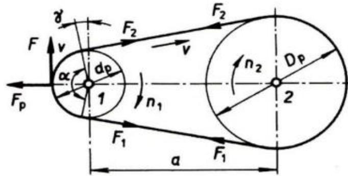
Fig. 1. Force ratio in the belt gear
