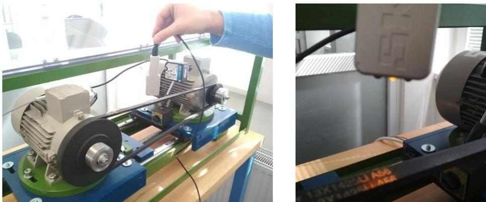
Fig. 5. Adjustment and tightening of the belt by means of contactless belt tension meter SKF
